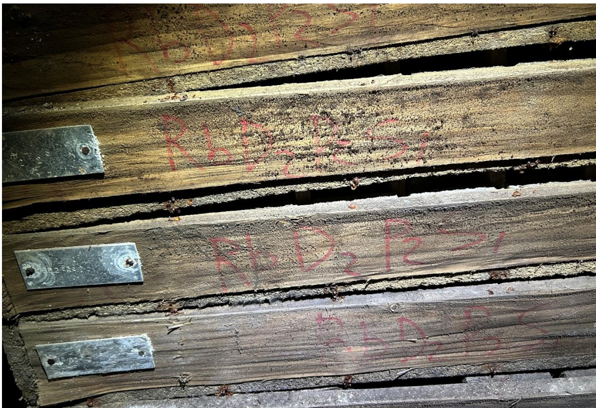
Figure 10.8: Core boxes showing hole names in development drive LRbRT37 (source: AMS site visit, 2026).
