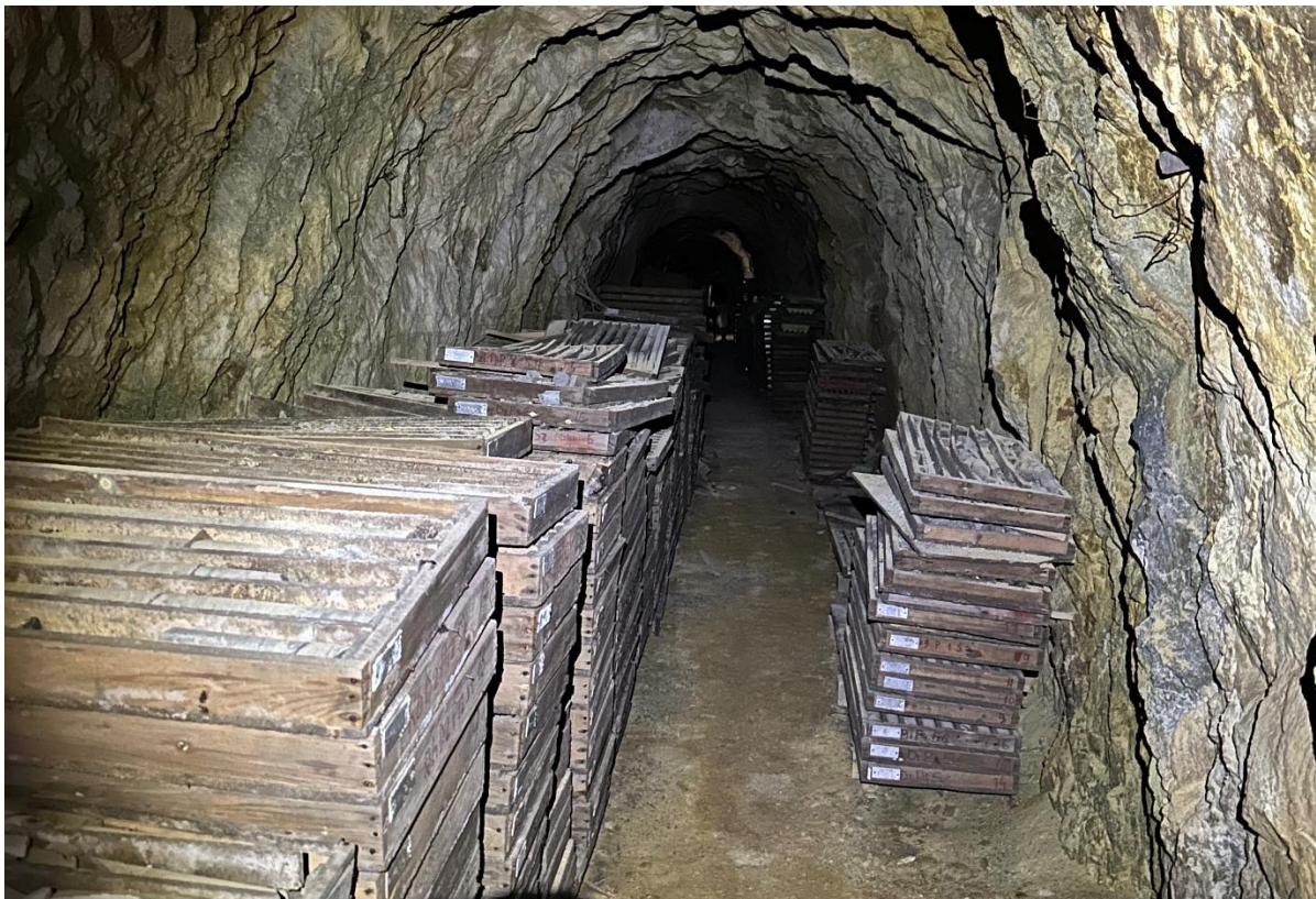
Figure 10.6: Reasonably well preserved core in development drive LRbRT37 (source: AMS site visit, 2026).
